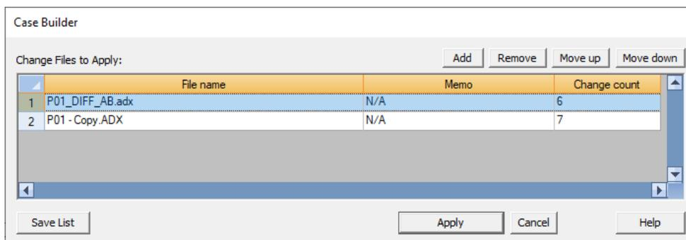
To apply the same set of change files to a difference base case, you can simply run the Case Builder command and open that .CBX file that you have saved previously.
