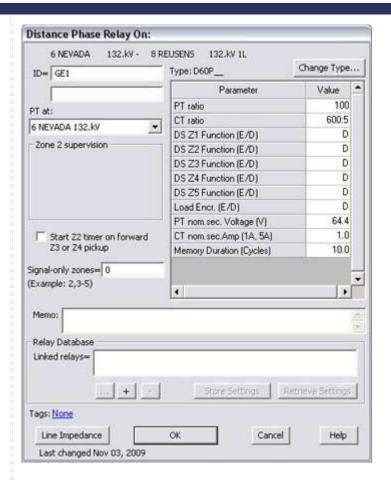
Fig. 1a: Info dialog box for a GE D60 relay, when all the zones are disabled.
