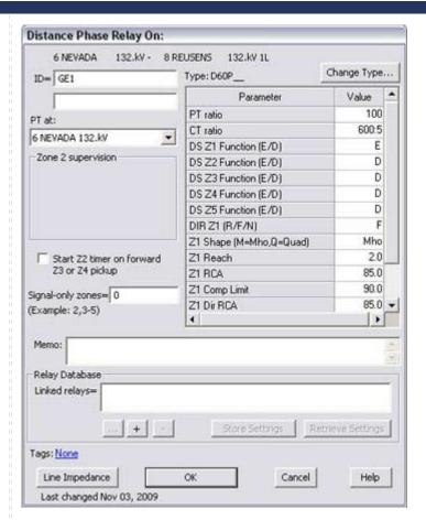
Fig. 1b: Info dialog box for a GE D60 relay, after zone 1 is enabled.
